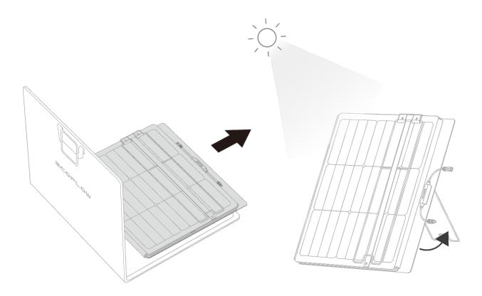
2 As shown in the picture, it's recommended to unfold the bracket first before unfolding the panel.
