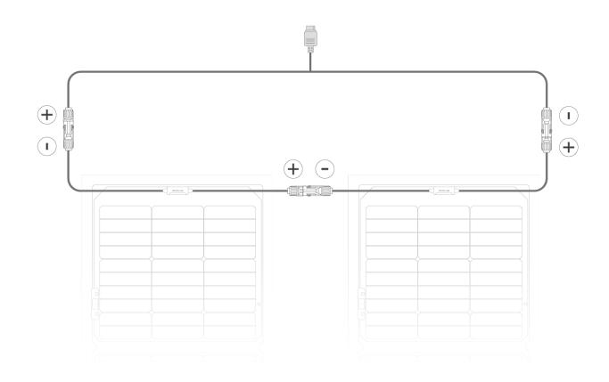
To wire **in parallel**, connect all positive ends of the panels' output cables to a solar parallel connection cable, and do the same for the negative ends. Then, connect the solar to XT60i charging cable to the solar parallel connection cables. When connecting, refer to the instruction images to avoid misconnecting the male and female connectors of the parallel connection cables.
