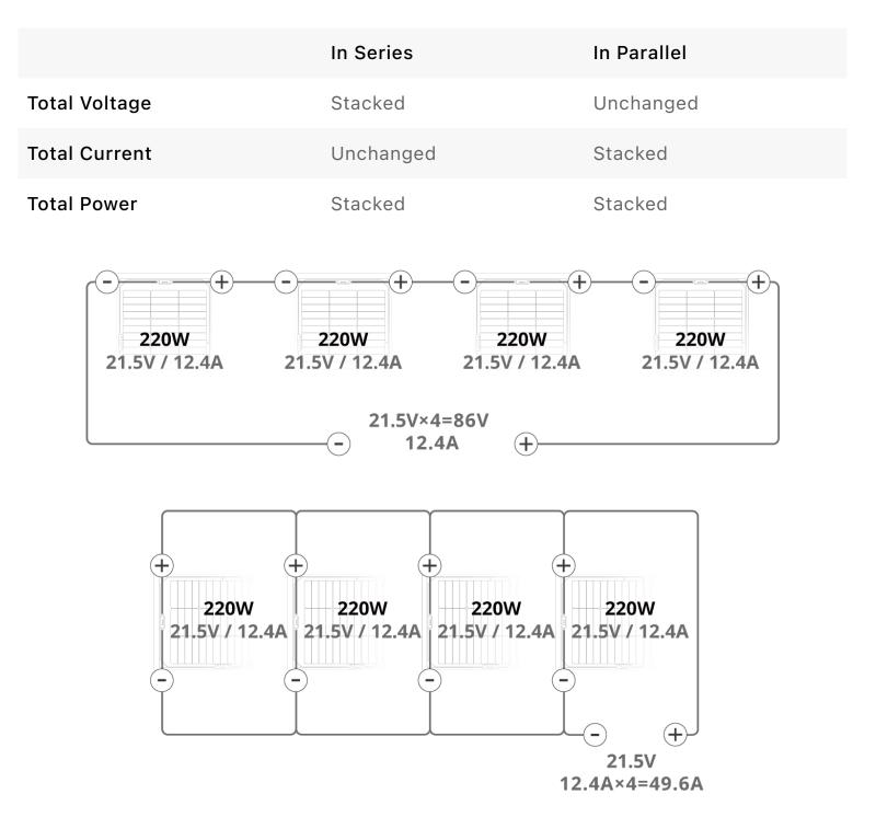
• Solar panel wiring of different ratings
