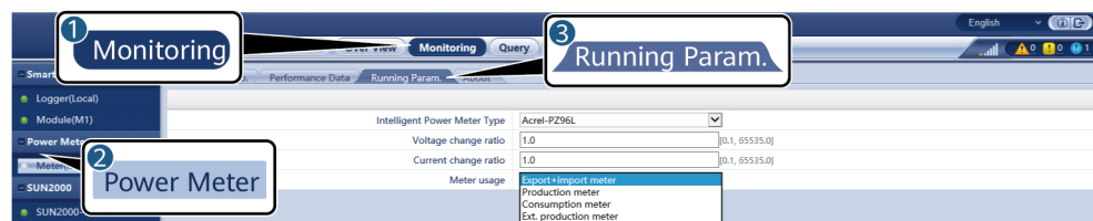
Figure 6-33 Setting power meter parameters
