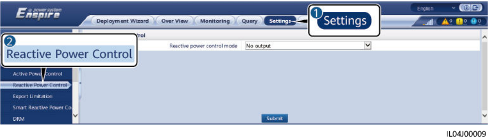
Figure 6-53 Reactive power control
