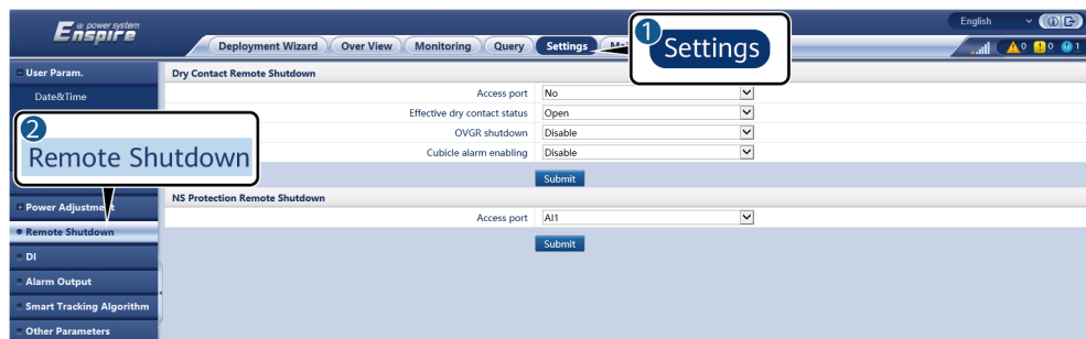
Figure 6-65 NS protection remote shutdown
