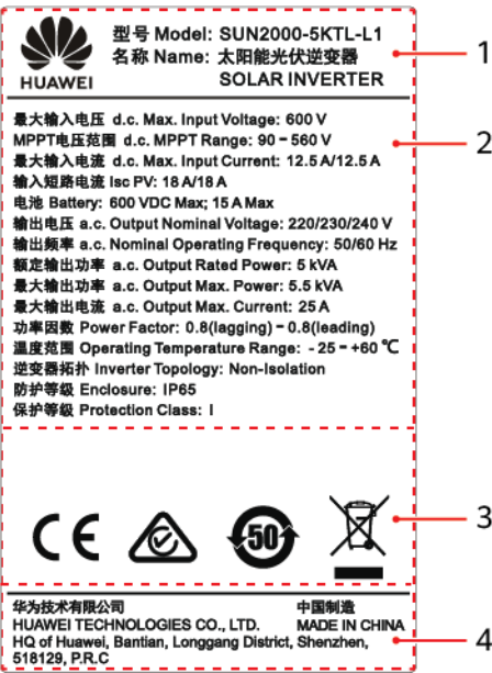
Figure 2-7 Nameplate (using SUN2000-5KTL-L1 as an example)
