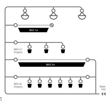
KIT REQUIRED: SOL-C24L, 12 Dripper Ext kit, 12m Seep Hose Spare capacity: 6 Drippers
