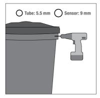
Connecting to the Water Barrel
