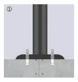
4. Install the gasket and tighten the nut.
