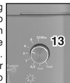
14. As soon as everything is assembled, please put the selector switch to the position „Test“. The pump will then start to work if the battery is charged sufficiently. The pump sucks in the water autonomously. In doing so, make sure that the filter of suction hose is below the water surface.
