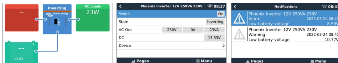
Example of GX screens from left to right: system screen, inverter device screen, and alarm message.
