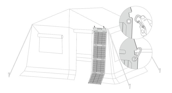
For long-term use, ensure that the panel is securely fixed to avoid falling off in windy conditions.
