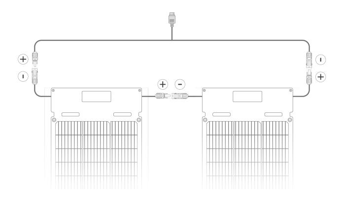
To wire **in parallel**, connect all positive ends of the panels' output cables to a **solar parallel connection cable**, and do the same for the negative ends. Then, connect the **solar to XT60i charging cable** to the solar parallel connection cables. When connecting, refer to the instruction images to avoid misconnecting the male and female connectors of the parallel connection cables.
