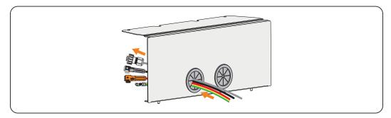
Figure 6-26 Threading cables
