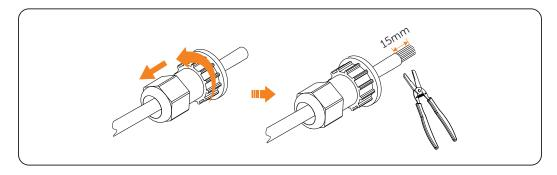
Figure 7-23 Stripping cable jacket
