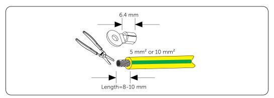
Figure 6-17 Striping cable jacket
