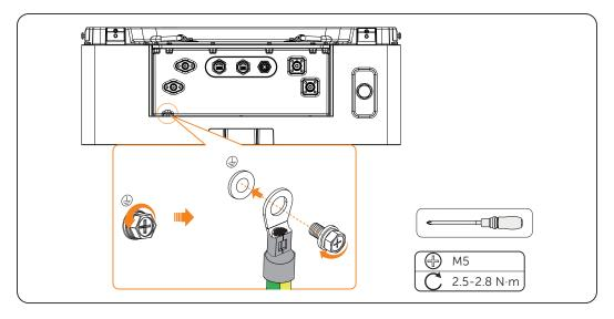
Figure 6-20 Tightening M5 screw
