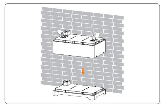
Figure 7-6 Placing battery pack
