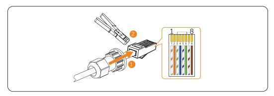
Figure 7-24 Crimping RJ45
