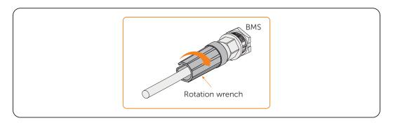
Figure 6-30 Closing communication cable
