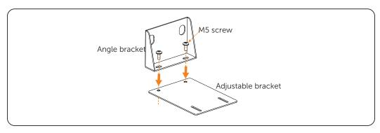
Figure 7-9 Assembling bracket
