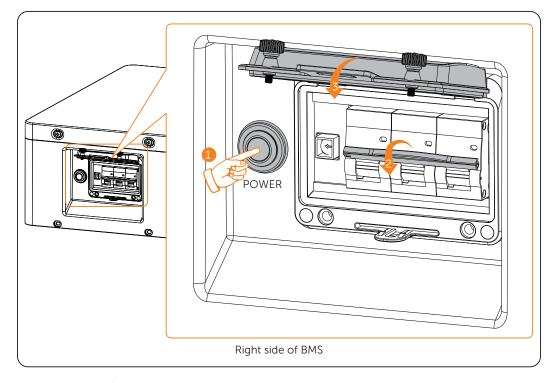
Figure 8-4 Pressing the button and flipping down the breaker
