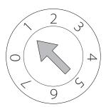
Figure 2-2 DIP switch: "1" position
