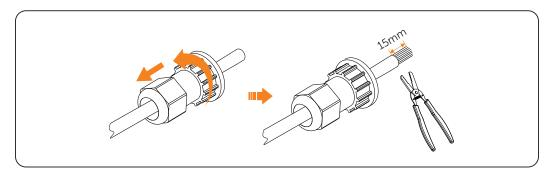
Figure 6-22 Stripping cable jacket
