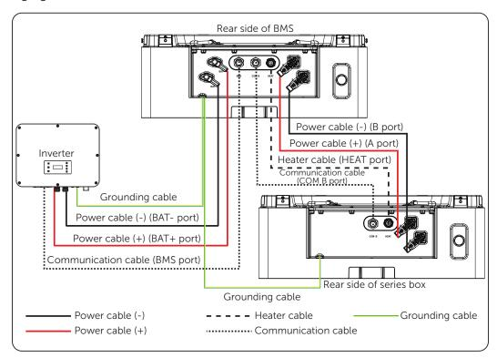
Figure 7-17 Wiring diagram
