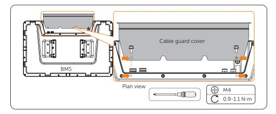
Figure 6-32 Tightening M4 screw
