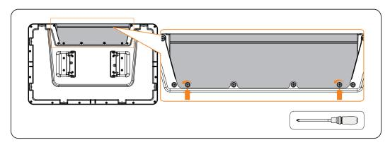
Figure 9-4 Removing cable guard cover
