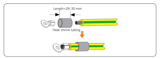
Figure 7-19 Cutting heat-shrink tubing
