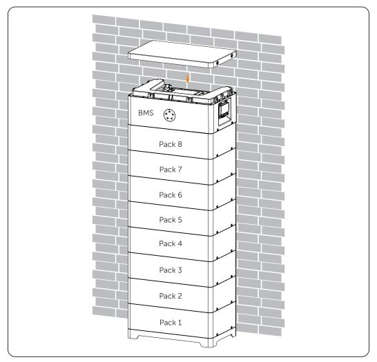
Figure 6-34 Placing BMS
