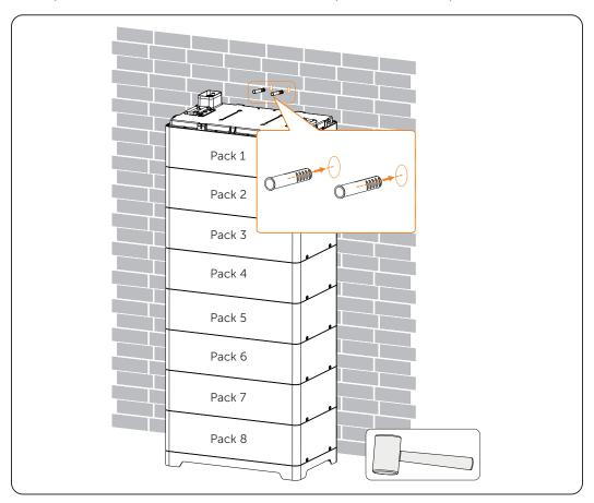
Figure 6-12 Inserting expansion bolt
