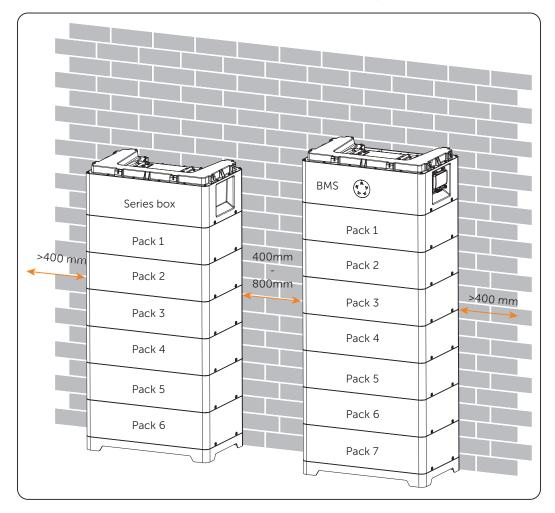
Step 13: Repeat steps 1 to 12 to install the remaining battery packs and series box.
