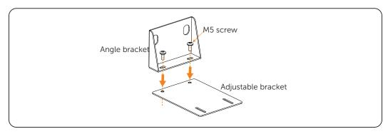
Figure 6-9 Assembling bracket
