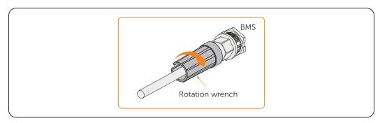
Figure 7-37 Closing communication cable
