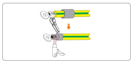
Figure 7-20 Crimping and heating
