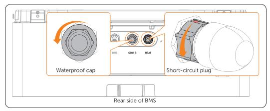
Figure 7-28 Removing waterproof cap and short-circuit plug
