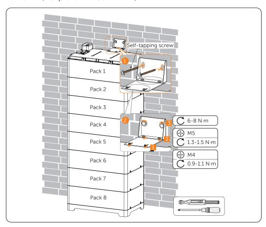
Figure 7-13 Securing assembled bracket
