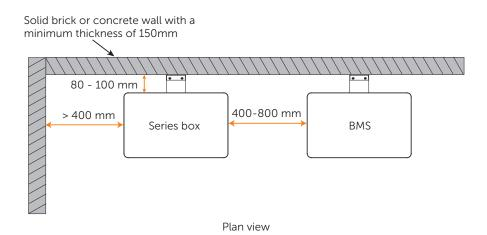
Figure 4-4 Installation clearance for two towers
