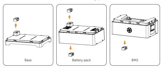
Figure 7-2 Removing dust cover
