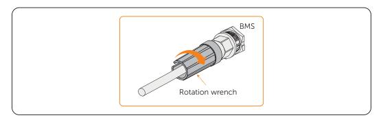
Figure 7-32 Closing communication cable
