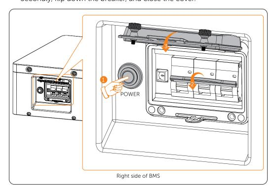
Figure 9-2 Pressing the button and flipping down the breaker
