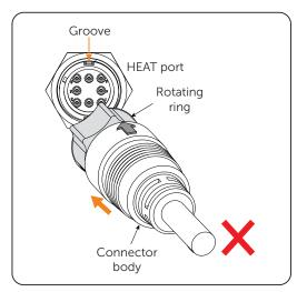
Figure 7-34 Plugging heater cable
