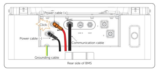
Figure 7-31 Connecting cables to inverter
