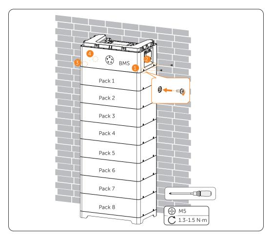
Figure 6-15 Tightening M5 screw
