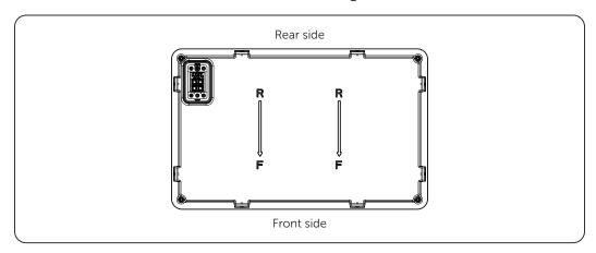
Figure 6-3 Placing base
