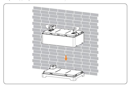
Figure 6-6 Placing battery pack
