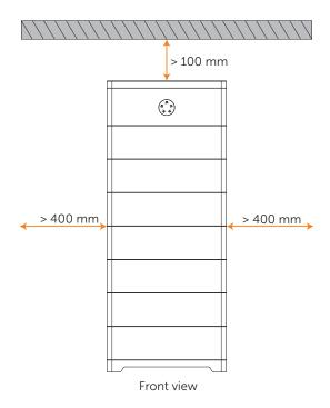
Figure 4-2 Installation clearance for one tower
