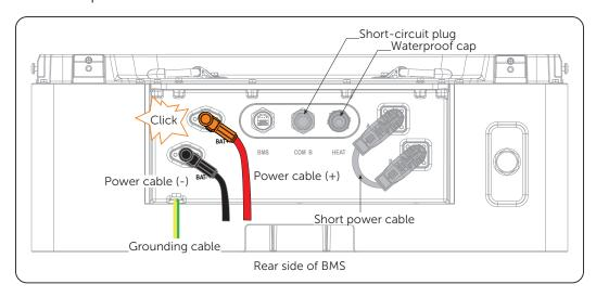
Figure 6-27 Plugging power cables
