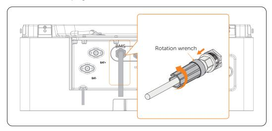
Figure 11-5 Unplugging communication cable
