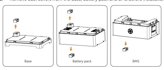
Figure 6-2 Removing dust cover
