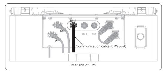
Figure 6-29 Plugging communication cable
