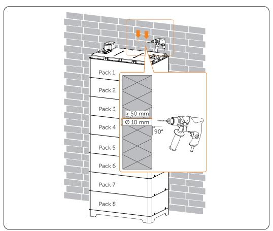
Step 9: Remove the assembled bracket, and drill holes. (Drill bit:  $\emptyset$  10mm; Drill depth:  $\ge$  50 mm)
