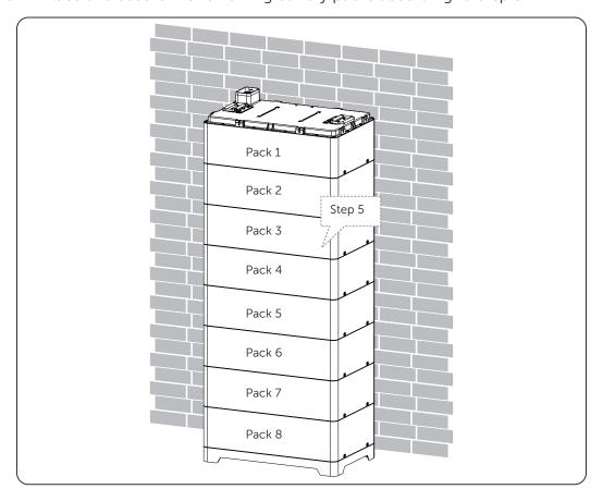
Figure 6-8 Placing battery pack
