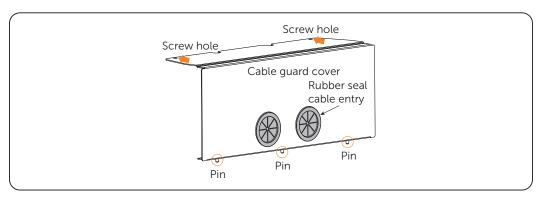
Figure 7-29 Details of cable guard cover
