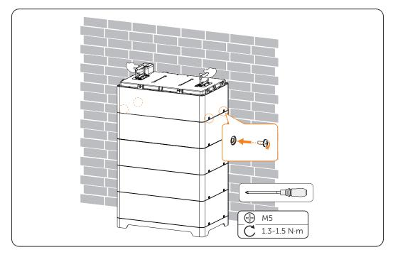
Figure 9-12 Placing battery pack and securing M5 screw
