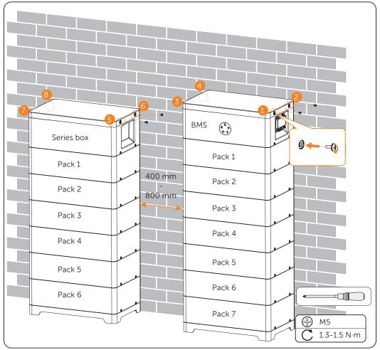
Figure 7-43 Tightening M5 screw
