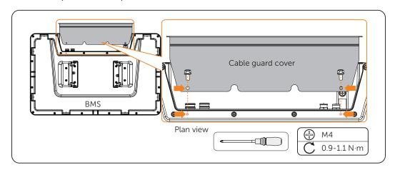
Figure 7-40 Tightening M4 screw
