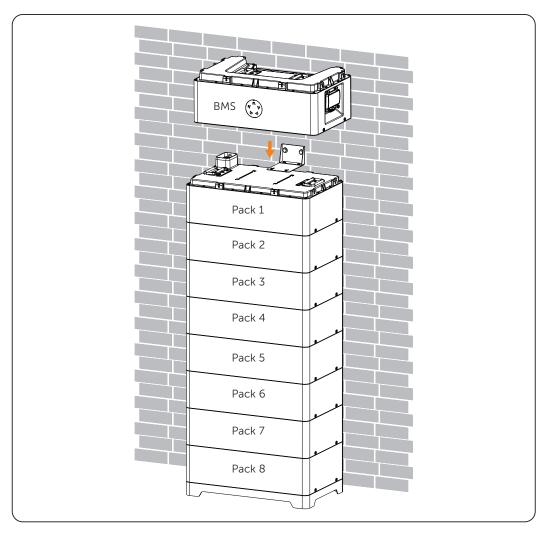
Figure 7-14 Placing BMS
