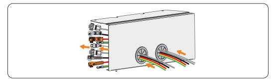
Figure 7-30 Threading cables
