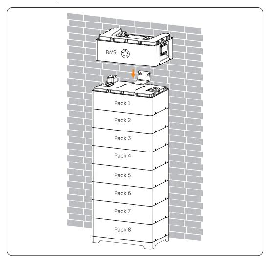
Figure 6-14 Placing BMS
