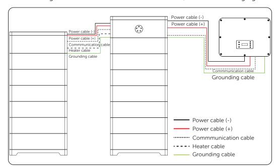
The installation diagram about two towers with an inverter, see the following figure:
