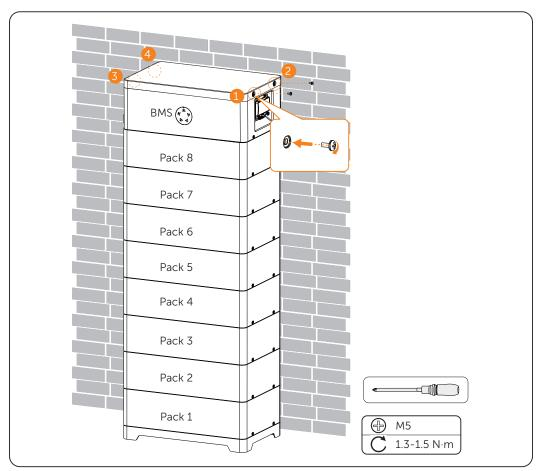
**Step 10**: Correctly insert and tighten the M5\*14 Phillips cheese head screw (Part F) to secure the base and battery pack. (M5: 4 pieces) (Torque for M5: 1.3-1.5 N·m)
