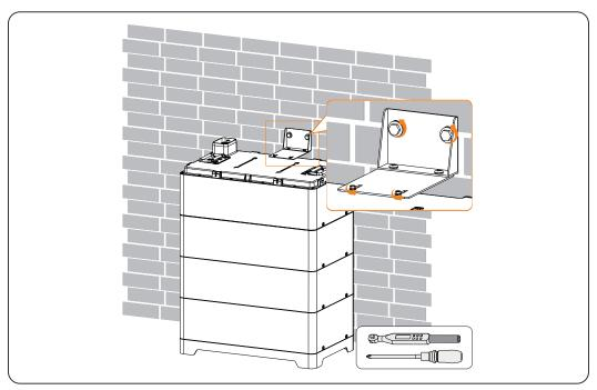
Figure 9-11 Removing assembled bracket
