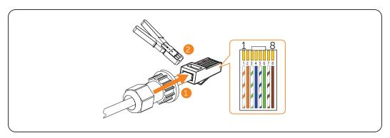
Figure 6-23 Crimping RJ45
