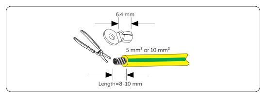
Figure 7-18 Striping cable jacket
