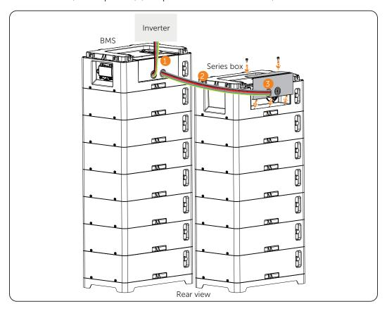
Figure 7-41 Pulling cables and securing cover
