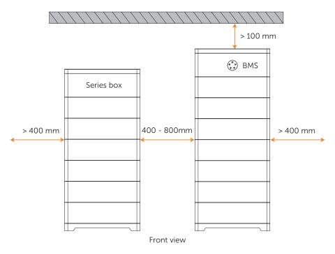
Figure 4-3 Installation clearance for two towers
