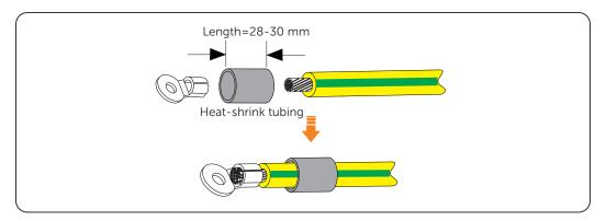
Figure 6-18 Cutting heat-shrink tubing
