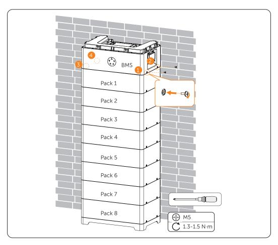
Figure 7-15 Tightening M5 screw
