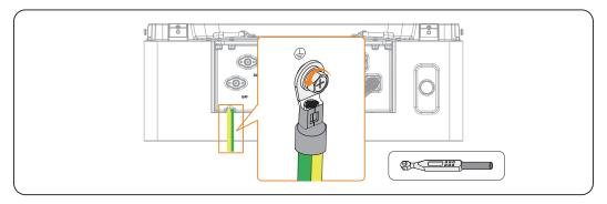
Figure 11-6 Disassembling grounding cable
