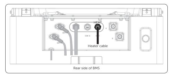
Figure 7-35 Diagram after installation of heater cable
