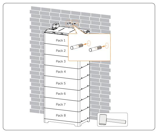
Figure 7-12 Inserting expansion bolt
