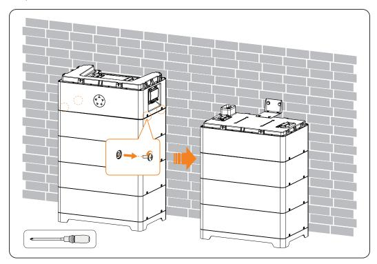
Figure 9-10 Removing BMS
