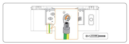
Figure 9-9 Disassembling grounding cable
