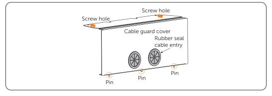
Figure 6-25 Details of cable guard cover
