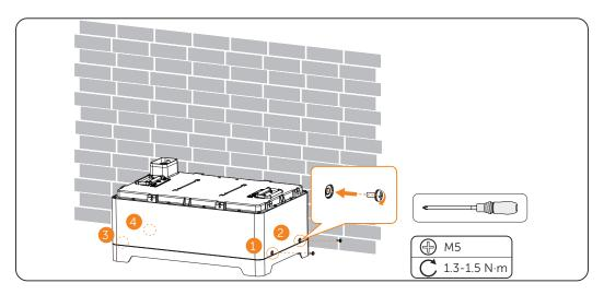
Figure 6-7 Tightening screw
