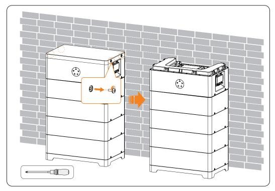
Figure 9-3 Removing BMS cover
