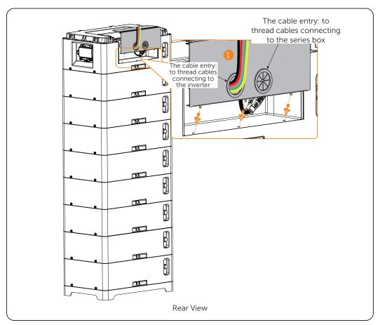
Figure 6-31 Inserting cable guard cover
