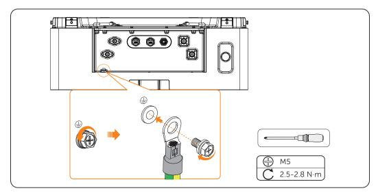
Figure 7-21 Tightening M5 screw
