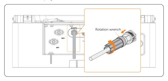
Figure 9-8 Unplugging communication cable
