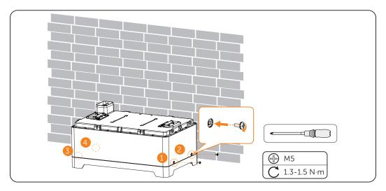
Figure 7-7 Tightening screw
