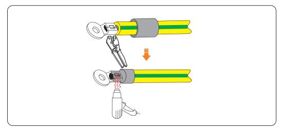
Figure 6-19 Crimping and heating
