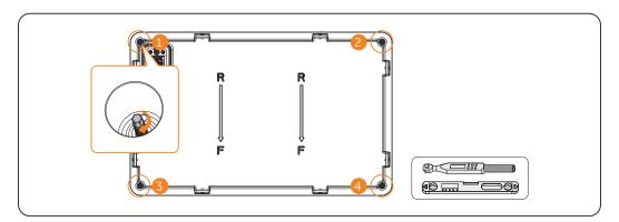
Figure 6-4 Rotating adjustable screw
