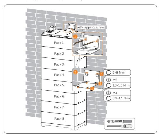
Figure 6-13 Securing assembled bracket
