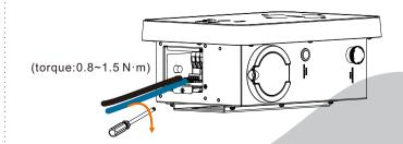
STEP 11: Push the rear cover to appropriate position of the cables and screw the self tapping screws with the cross screwdriver. Then tighten the waterproof fastening head.
